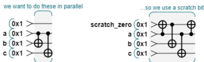
In this example, our operation didn't get any faster, because we ended up with four gates, and only two can be run in parallel. In practice, we can probably do the scratch-prep well in advance (and usually in parallel with some other operation), so we'll often get it for free. In fact, when we need many of these scratch bits at once, we can use them to create more, like zombies and vampires.
