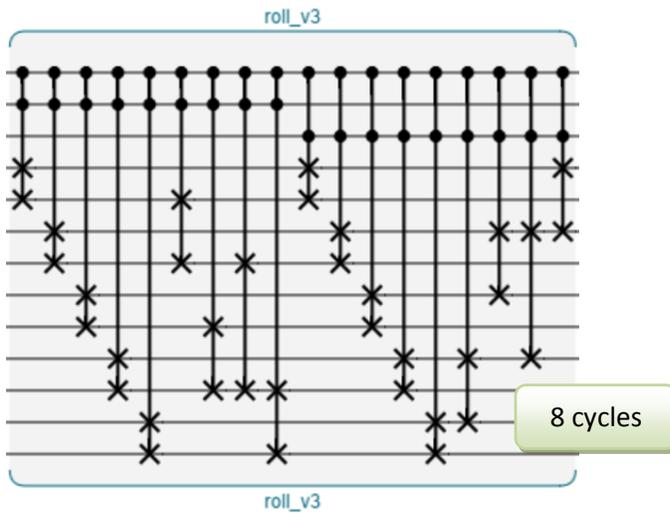
...so why bother with this? Two reasons. First, those first five gates are now identical, and first, so we can simply use a single set of them for both forward and backward. Second, *none* of the remaining gates actually overlap between the forward and reverse directions. So if we interleave them, they can be done in parallel.
