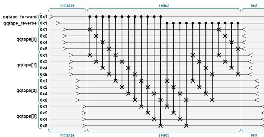
Note that since the forward and reverse controls are themselves qubits, this machine is capable of traveling forward *and* reverse *and* staying still, all at once. Here’s one which uses 16 bytes of 8 bits each (this requires 132 qubits total, and 240 gates, but it can be done in 30 cycles because each byte’s bits are taken in parallel on the hardware.):
