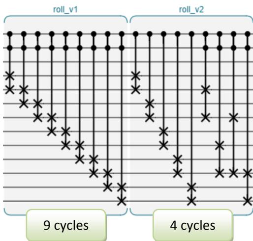
The first method (roll\_v1) requires 9 gates, and each must be completed before the next can begin, because their target qubits overlap. So this will take 10 cycles (at least) on actual QC hardware.
