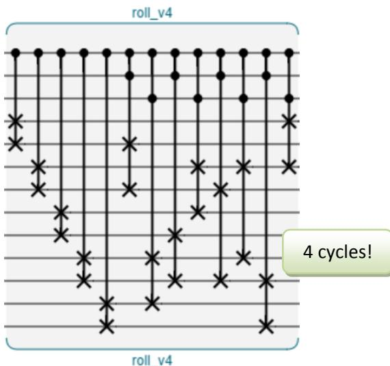
There's one limitation, which is that the QQTape length must be an even number. Going from 18 cycles to 4 is a massive speedup, but it gets better as this device grows in complexity. For  $n$  bytes, the original version requires  $2 \cdot (n - 1)$  cycles to execute. Our new version runs in something like  $\log_2(n)$  cycles. So for a 100-byte QQTape, instead of 198 cycles, we're looking at about 7. That's why we did this.
