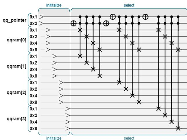
The **initialize** operation simply writes the initial values. After that, we can use the **select** operation to swap location qqram[0] with whatever location is pointed to by qq\_pointer. So **select** is essentially a "fetch", and we can think of qqram[0] as the register we're fetching into. The critical feature is that if qq\_pointer is a superposition of multiple values, then multiple locations will be fetched at once.
